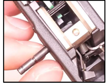
Step 36: Use your Micro-Tip to Maneuver the Slide Stop until the Trigger Hinge Pin has Clearance
