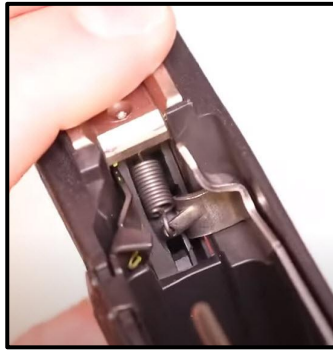
Step 34: Check that the Slide Stop Spring Leg is sitting on top of the Slide Stop.
