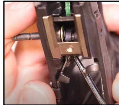
Step 36: Use your Micro-Tip to Maneuver the Slide Stop until the Trigger Hinge Pin has Clearance
