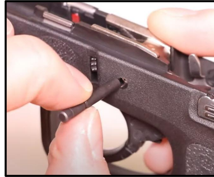
Step 36: Use your Micro-Tip to Maneuver the Slide Stop until the Trigger Hinge Pin has Clearance
